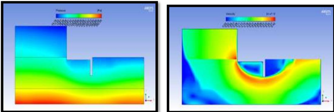
**Fig.4-8: case 3 pressure and velocity contour with angle 90 degree.**
