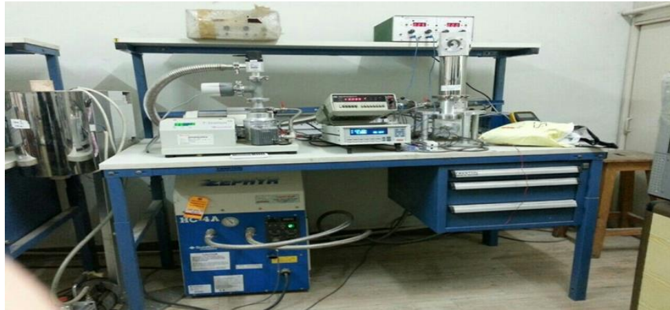
Figure (3) Voltage and current difference measurement system for samples at low temperatures.
