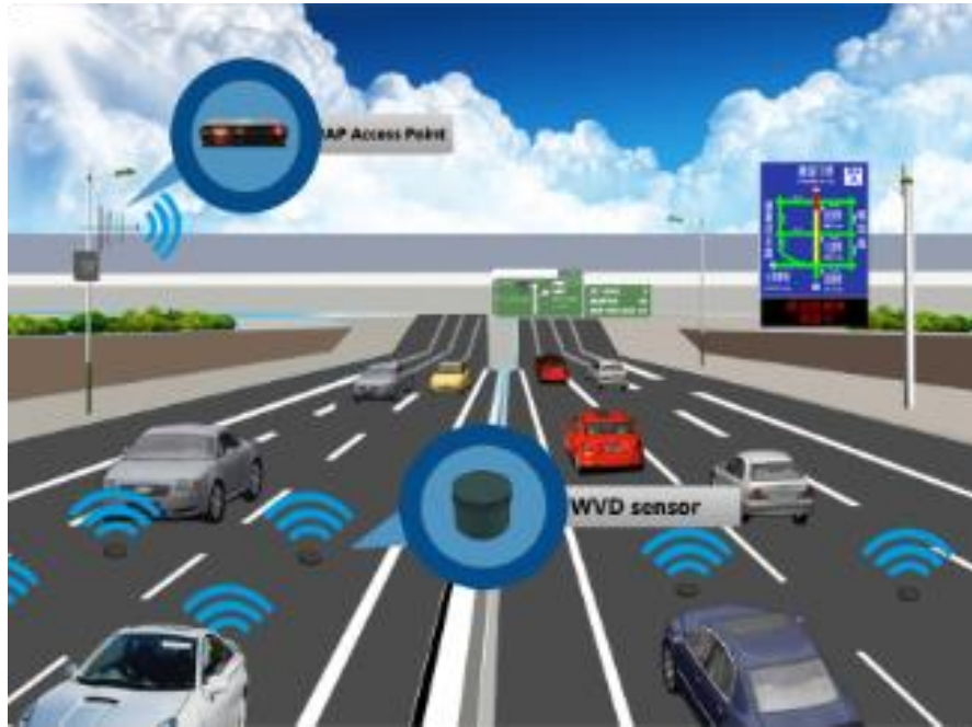
Figure 5: Sensors that count the number of passing vehicles through a street.
