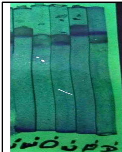
Fig(4): shows SDS gel electrophoresis of the standard protein with purified Bromelain the tubes from left to right contained (25)µg of standard protein employed to calibrate the columns were :a. Bromelain purified b. Urease (M.wt.480000)c. Egg albumin (M.wt.45000).Pepsin (M.WT.36000).e. Bovin serum albumin (BSA) 67000.
