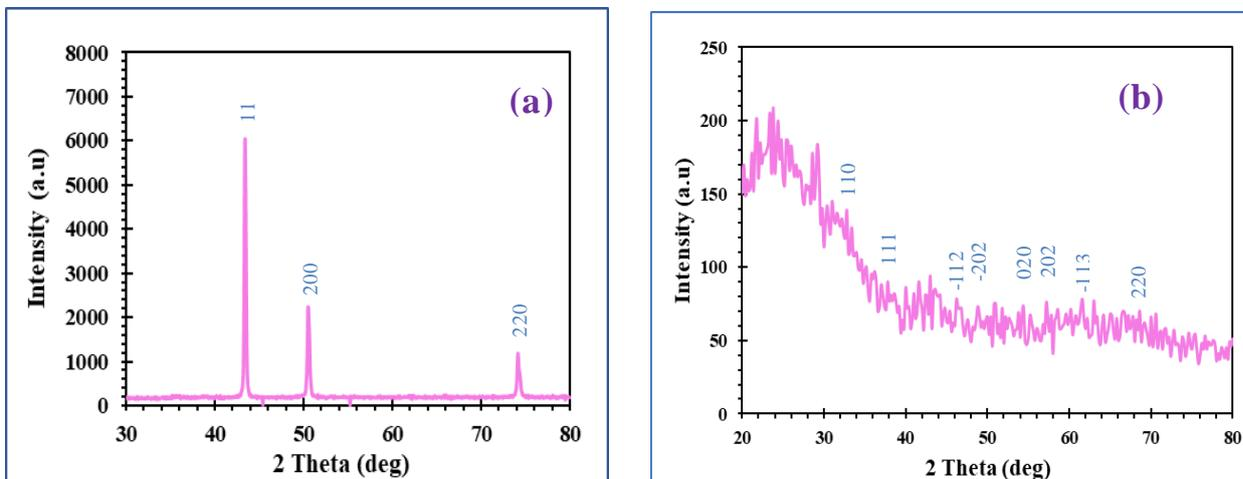
Figure -4 XRD patterns of (a) pure copper powder (b) XRD pattern of CuO
