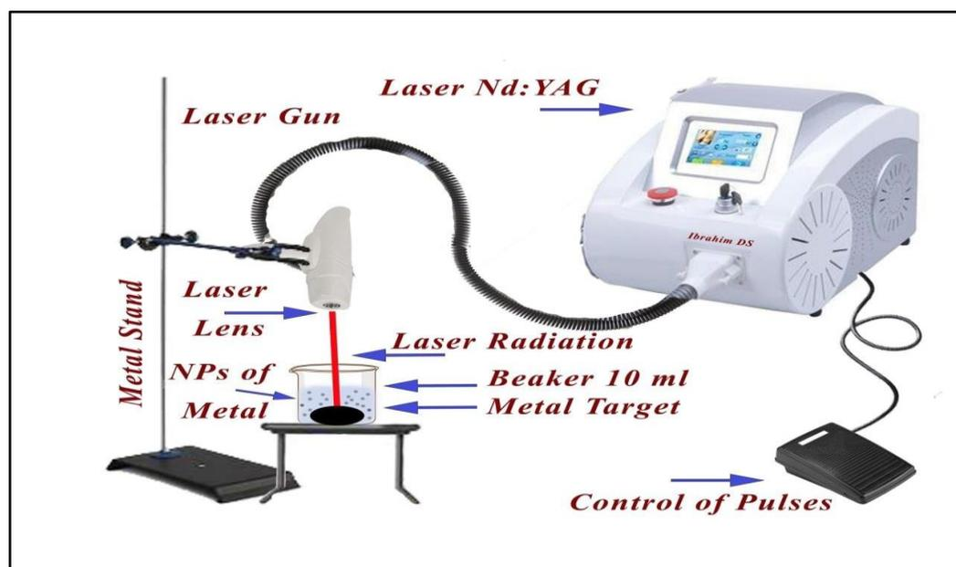
Figure -1 Experimental setup Laser ablation in liquid using Nd: YAG with  $\lambda=1064$  nm.
