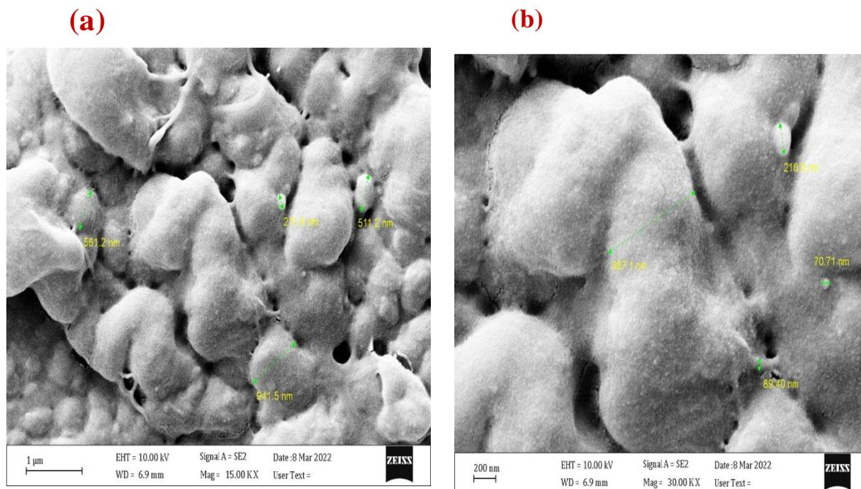
**Figure -5 FE-SEM images of CuO NPs measurement at range (a) 1 μm (b) 200 nm with laser energy 700mJ.**
