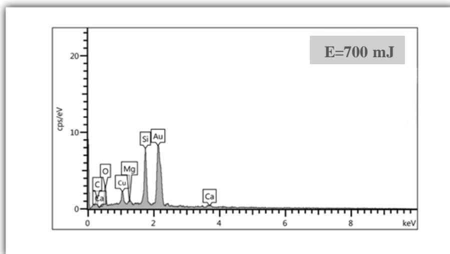
**Figure -6 The EDX pattern of CuO NPs at 700 mJ laser energy**
