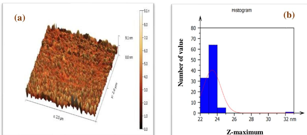
**Figure -7 (a) 3D AFM for CuO NPs prepared by PLA with 700 mJ laser energy
