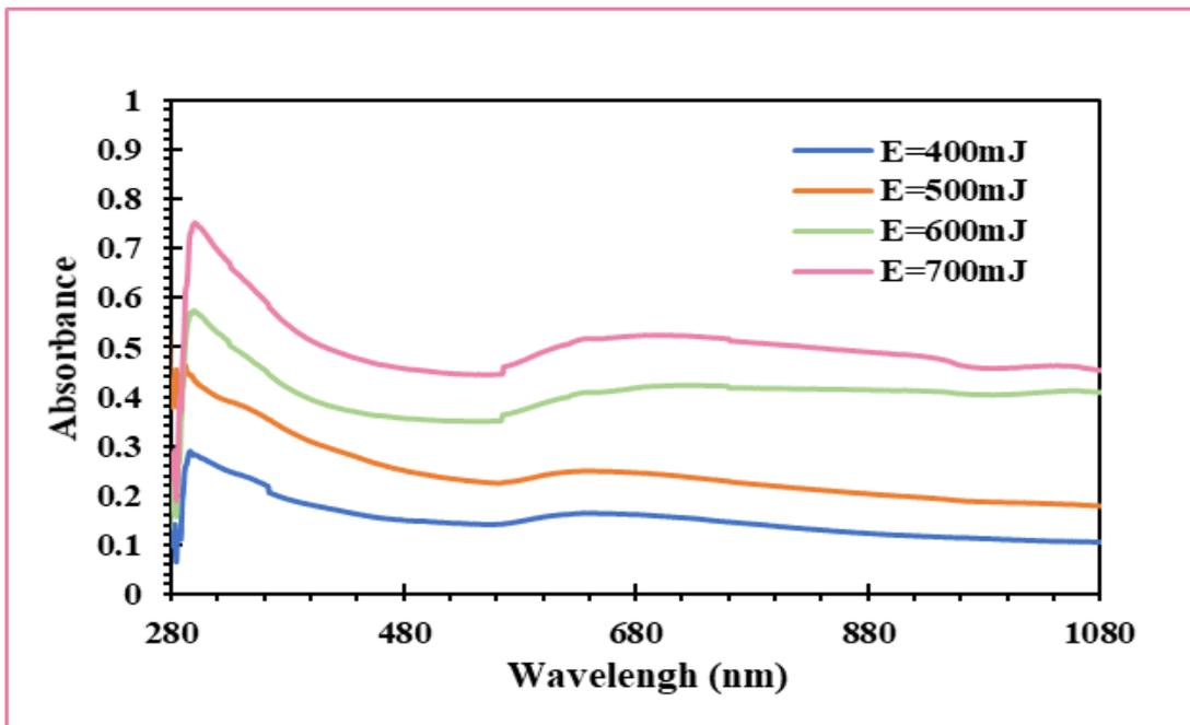
Figure -2 The absorbance spectrum as a function of the wavelength of the CuO NPs with different laser energy
