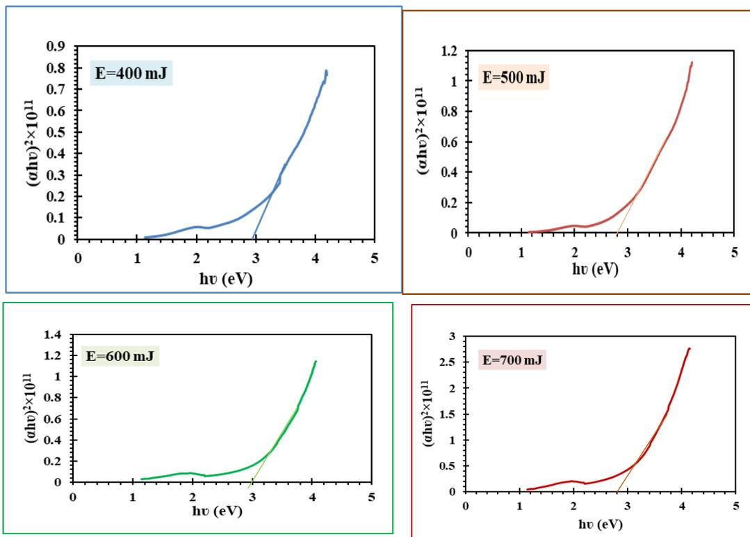
Figure -3 The relationship of  $(\alpha h\nu)^2$  as a function of the photon energy of the CuO NPs prepared by different laser energy.
