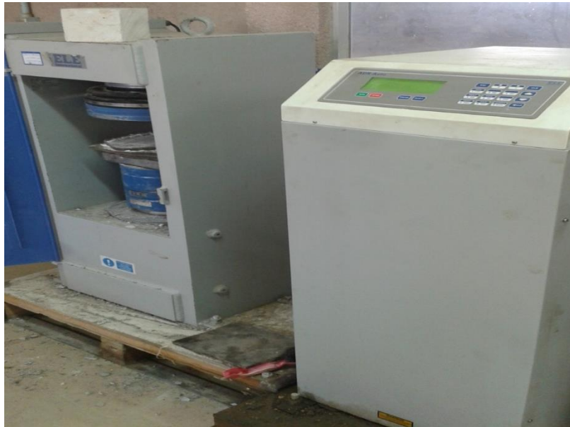
Figure (5) Compressive strength testing device used Resource: researchers
