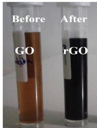
Figure 1: Photos of GO (left) and BrGO synthesized by Staphylococcus warneri (right) The UV-Vis peak of BrGO in Figure (2) shows maximum absorption of around 270 nm.
