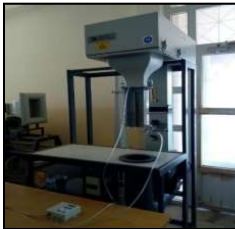
Figure(2): Air Flow Bench.
