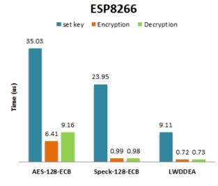
Figure 4. Run-time performance evaluation of AES, SPECK, and the proposed LWDDEA algorithm on NodeMCU ESP8266
